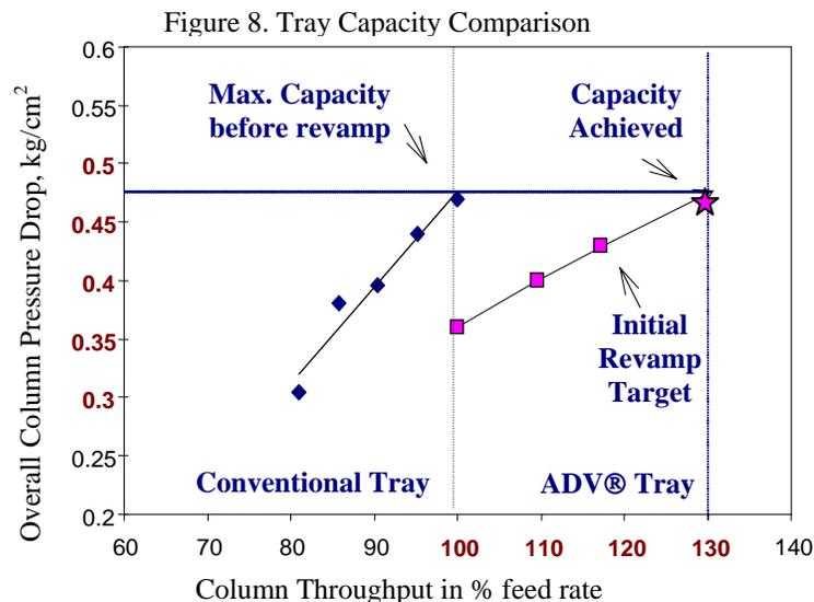
Table IV details the performance comparison before versus after revamp. It can be seen that Acetic Acid Dehydration Column with ADV<sup>®</sup> trays performed well with observed tray efficiency also higher than that of the original valve trays in the pre-revamp operation.
