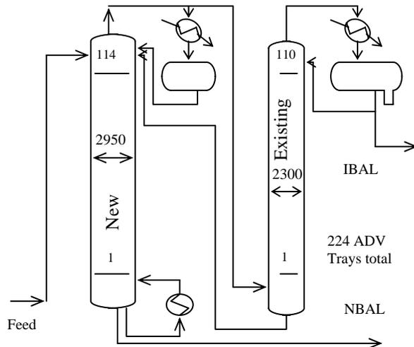
Fig. 10. Isomer Column (plant-1) PFD (after revamp)
