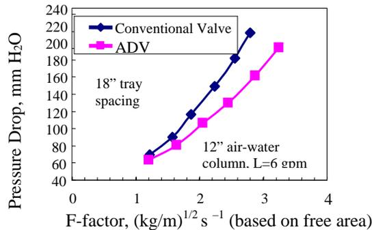
Figure 3. Pressure drop comparison
