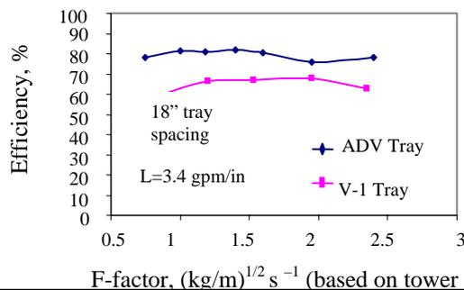
Figure 5. Comparison for valve tray
